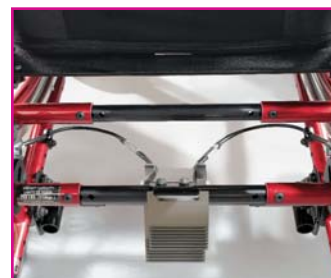
New heat-shrunk tubing around the hub lock cables along with an innovative foot-pedal assembly are designed to limit the cables from flexing further, improving durability.
