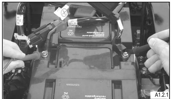
Note: To find a bad battery, use a battery load tester.
