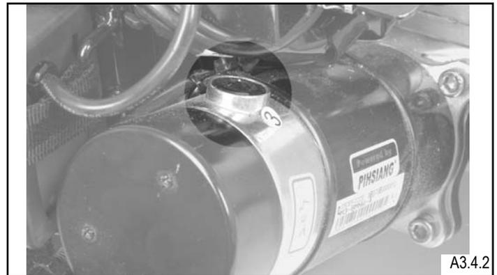
Use the meter to check the resistance across the two bottom contacts of the thicker wires on the 4-pin motor connector as shown in (figure A3.4.3). If the meter reads between 0 to 1.5 ohms, then replace the main harness. If none of the above corrects the problem, replace the right motor.
