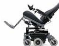
Major disadvantage is a tendency to “highcenter” – this means that with 6 wheels on the ground, the drive wheels can get stuck in the air when initiating a ramp or other obstacle. More and more mid wheel drive configurations offer different tracking and curb assist capabilities – while it is still not the best configuration for outdoors use, the performance constantly improves.
