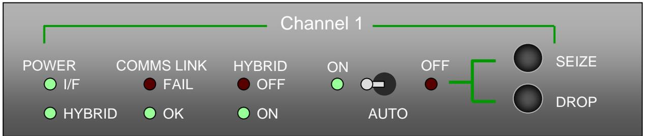
When in Auto mode, an incoming call will be answered with a blip of 2 tones being sent down the line. The tones are an indication to the caller to enter the Direct Dial DTMF tones, if required, to call an individual panel within the Telephone group. This feature is only available when the TIC card is installed. This is set up in the configuration software.
