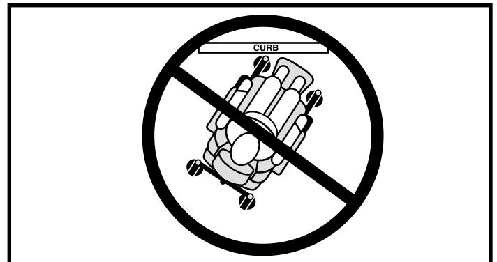
Figure 3. Incorrect Curb Approach
