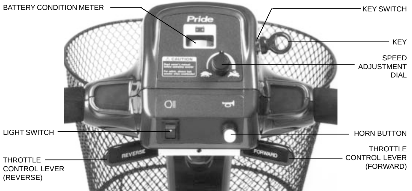
Figure 6. Control Console Assembly
