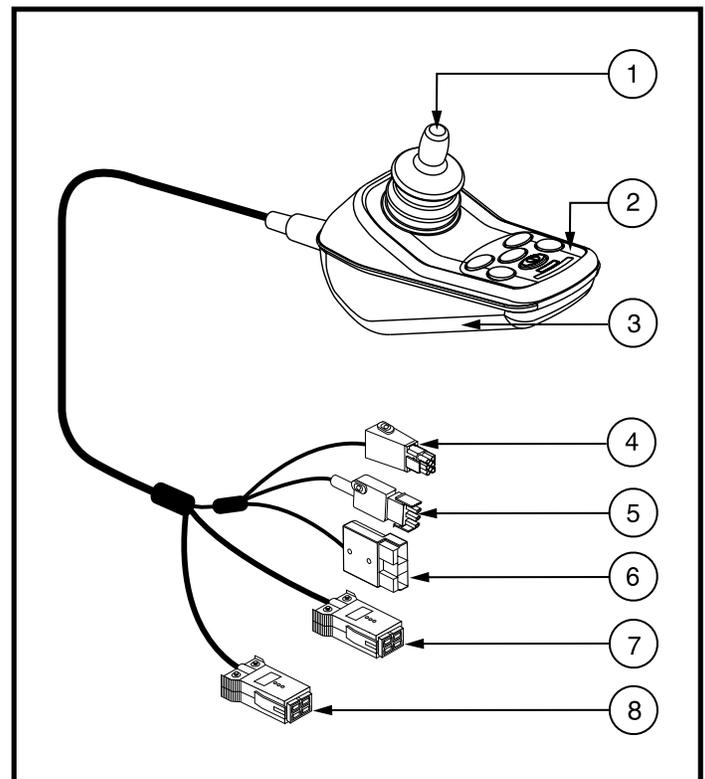
Figure 23. VSI Controller (Optional 6-key Shown)
