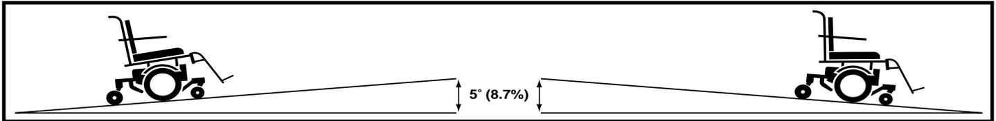
Figure 1. Maximum Safe Slope (Ascending and Descending)
