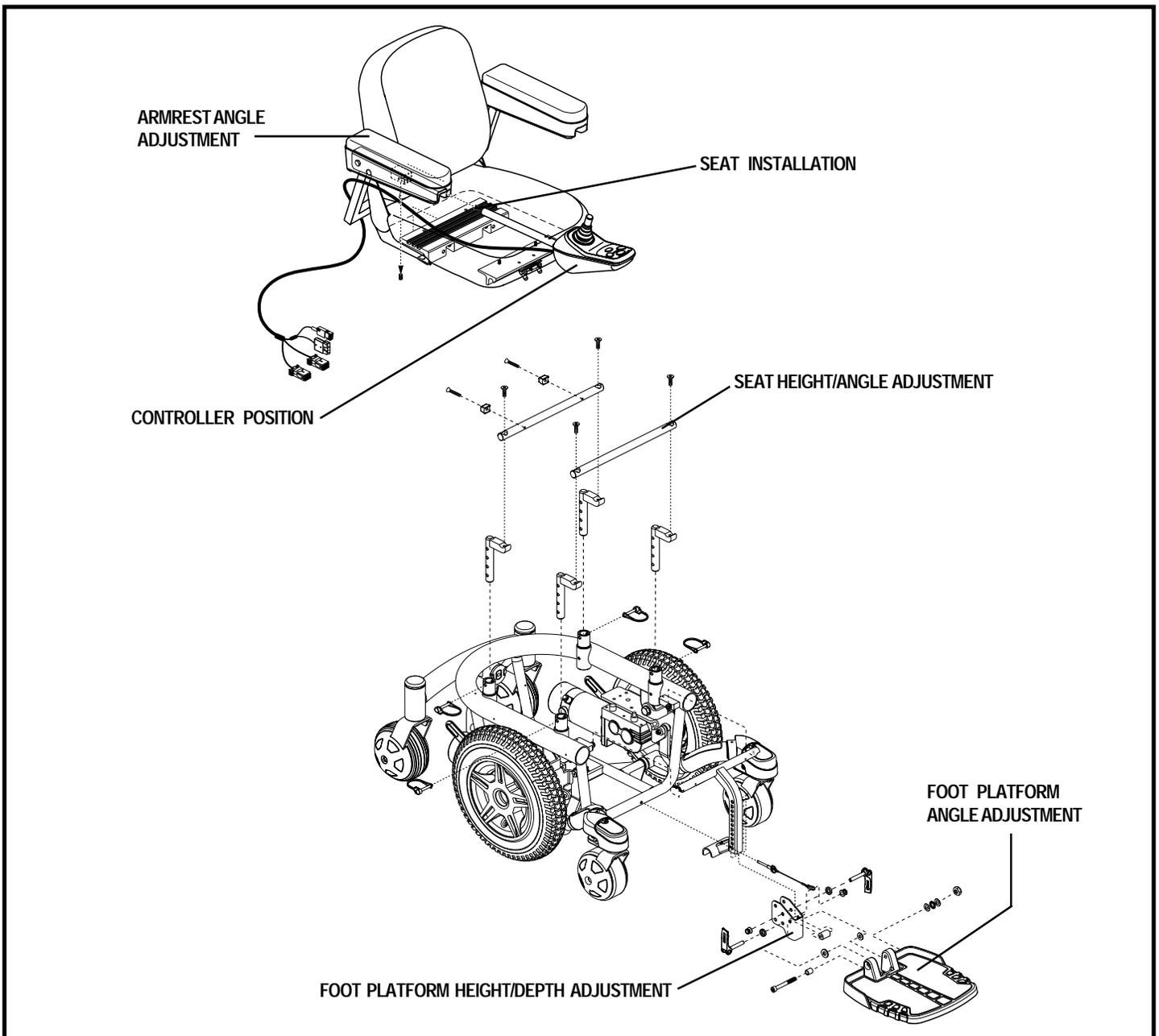
Figure 10. Quantum 600E Assembly View (Standard Seating Shown)
