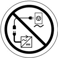
Prevent personal injury and equipment damage. Do not connect an extension cord to the AC/DC converter or the battery charger.
