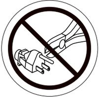
**Removal of grounding prong can create electrical hazard. If necessary, properly install an approved 3-pronged adapter to an electrical outlet having 2-pronged plug access.**
