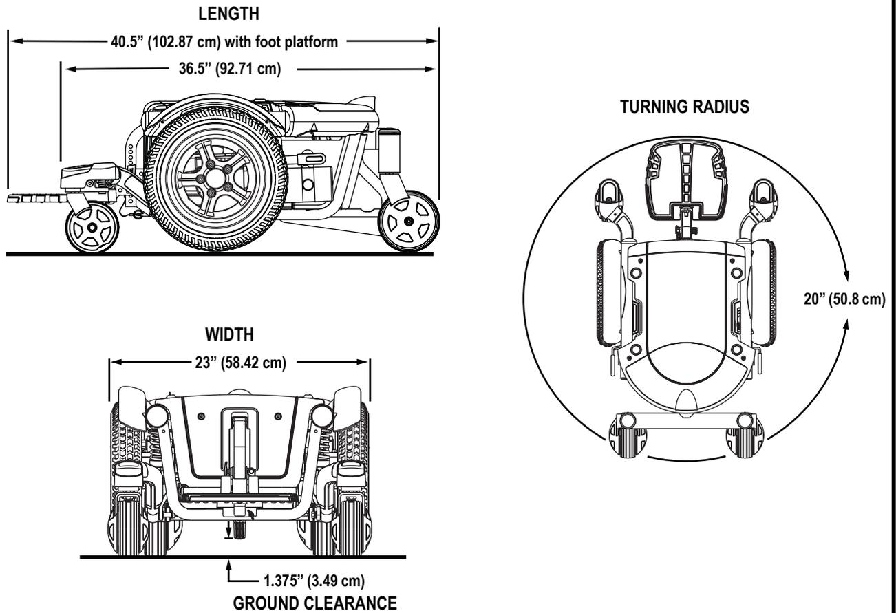
Figure 28. Quantum 600 Series Dimensions and Ground Clearance
