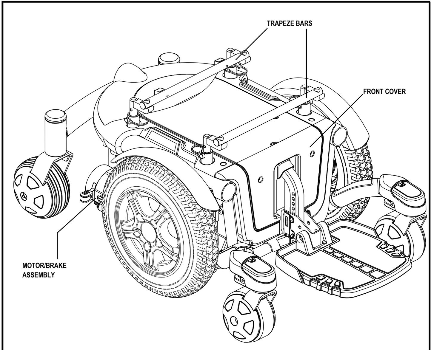
Figure 6. The Quantum 600 Series Power Base
