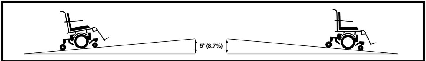
Figure 1. Maximum Safe Slope (Ascending and Descending)
