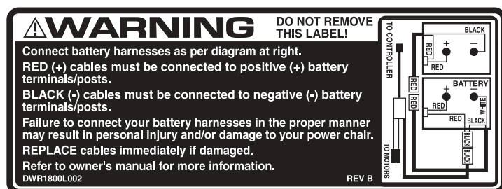
Figure 32. Battery Wiring Label
