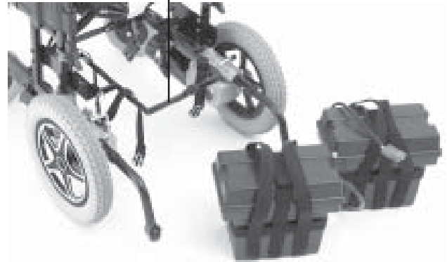
Figure 25. Pride LX - Battery Boxes Removed
