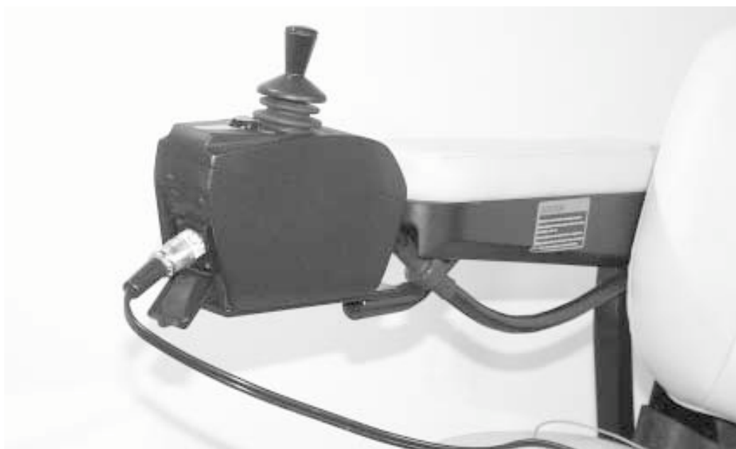
FIGURE 11. 3-Pin Charger Lead Plugged into the Joystick Programming Port
