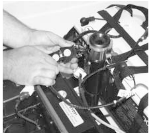
Figure 21. Connect Motor Harness Plug
