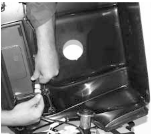
Figure 22. Connect Rear Light Harness
