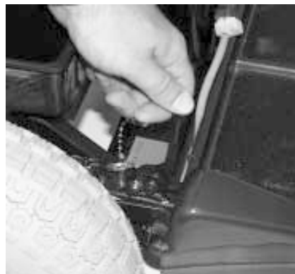
Figure 17. Push the Locking Cam Levers
