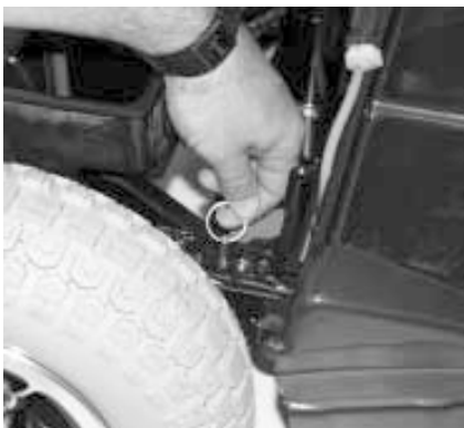
Figure 16. Secure Sections with Ball Detent Pins
