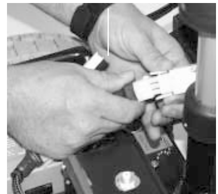
Figure 18. Plug in the 9-pin Connector
