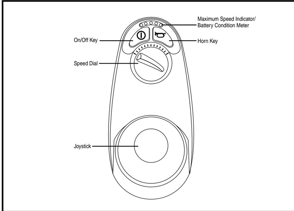
**Figure 3. Controller Keypad**
