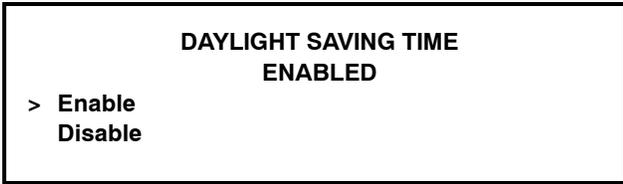
Pressing the UP or DOWN arrow symbols will move the arrow to “Enable” or “Disable”. Pressing the SEL symbol next to “Disable” selects that option and returns to the Manager Menu. Pressing the SEL symbol next to “Enable” selects that option and displays the second screen.
