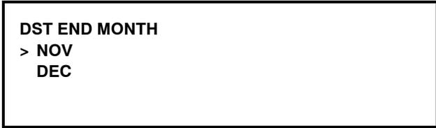
Pressing the SEL symbol next to the appropriate month will display the following screen. Press the UP or DOWN symbol to move the arrow to the appropriate week for the end of DST.
