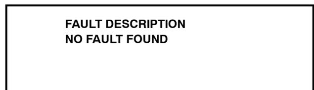
Touch the SEL symbol to display the next fault found or return to the Manager Menu if no other faults exist. Touching the SEL symbol any time faults are displayed will clear the faults, if corrected, upon returning to the Menu screen.
