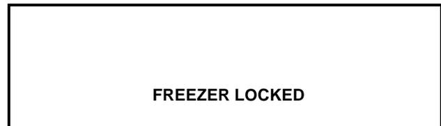
To restore the message that identified the reason for the hard lock, turn the power switch OFF for five seconds and then return the power switch to the ON position. The original message with the reason for the Hard Lock will be displayed.
