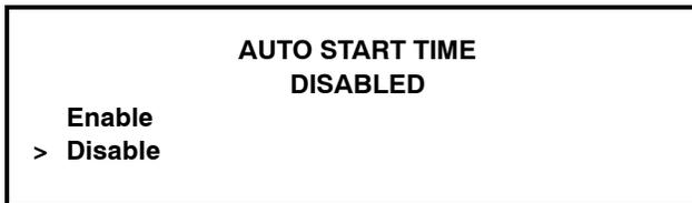
Enable the AUTO START TIME by touching the UP arrow symbol to move the arrow up to "Enable". Touch the SEL symbol to advance to the next screen.
