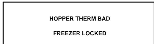
If the machine has hard locked and an attempt is made to enter AUTO, the machine will enter the STANDBY mode and display the following message.
