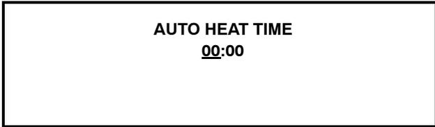
Touch the arrow symbols to increase or decrease the hour to the desired setting. Then move the cursor to the minutes position by touching the SEL symbol. Adjust the setting for minutes. Then touch the SEL symbol to save the setting and return to the AUTO HEAT TIME screen. Touch the SEL symbol to exit the screen and return to the Menu.
