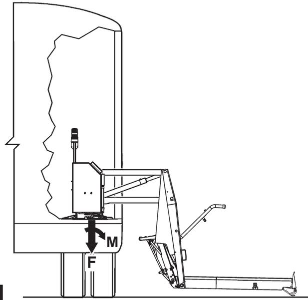
**FORCE & MOMENT PRODUCED BY LIFT ON VEHICLE FLOOR**
