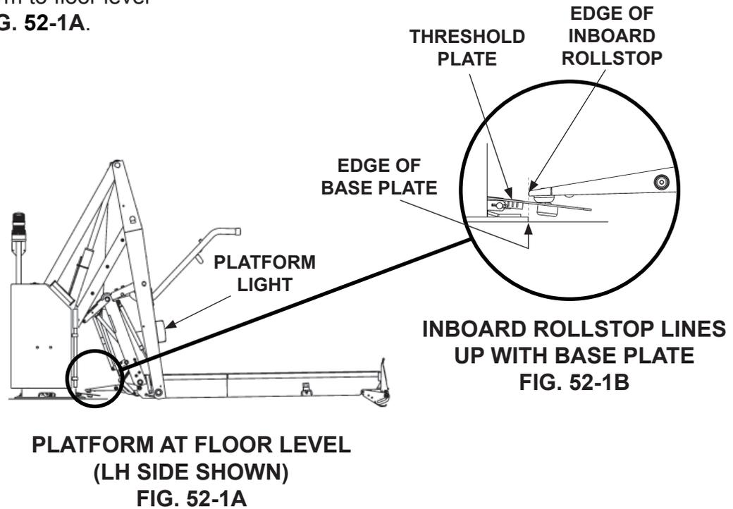
2. Inspect the threshold plate. The edge of the inboard rollstop should line up with the edge of the base plate as shown in **FIG. 52-1B**.
