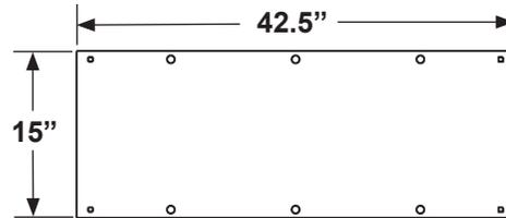
**LIFT FOOTPRINT ON VEHICLE FLOOR (LIFT WITH 33" OR 34" PLATFORM)**
