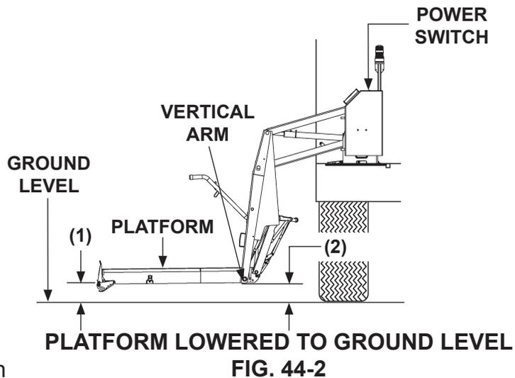
3. The measurement at the vertical arm (2) must be 1/2" - 1" more than the measurement at the front of platform (1). For example: If you measure 4" at the front (1), then you should measure from 4-1/2" to 5" at the vertical arm (2). If there is not a 1/2" - 1" difference, go to step 4 to obtain the correct measurement.
