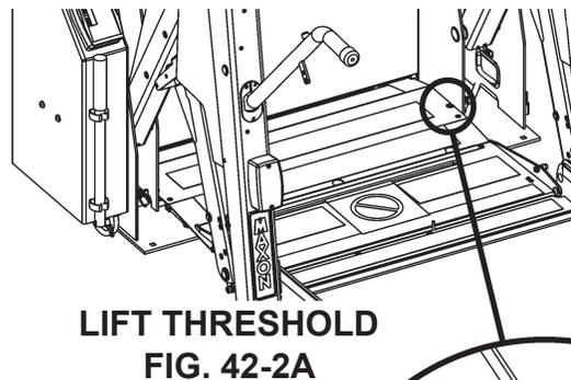
3. Set edge of the threshold plate to 5/8" height by turning the adjustment screw on the RH side of threshold plate (FIG. 42-2B). Turn adjustment screw counter-clockwise (FIG. 42-3) to raise threshold plate or clockwise to lower. Repeat for LH side of threshold plate. Alternately measure height (see instruction 2). Then, turn the adjustment screw on RH side and LH side until the entire edge of threshold plate is at 5/8" height.
