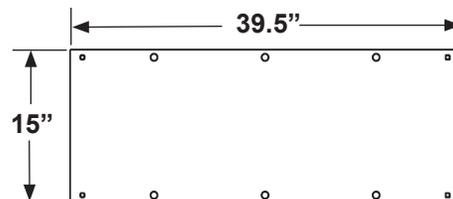
**LIFT FOOTPRINT ON VEHICLE FLOOR (LIFT WITH 30" PLATFORM)**
