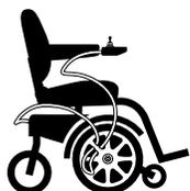
Use correct tie-down points for controller harness to prevent the harness from getting caught in the drive tires or pinched in the seat frame.
