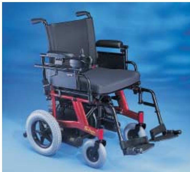
The R32 and R32Lx can be disassembled and folded for easy transport.
