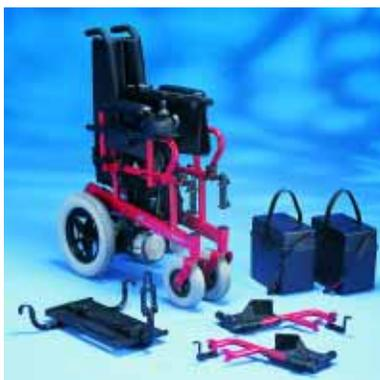
Components disassemble for easy transport
