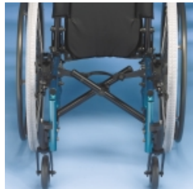
The Less-Seat-Rail option allows easy placement of seating systems.
