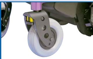
Utilizes elastomer dampeners that may be changed to provide dampening for all weight capabilities. Designed for 8" casters.
