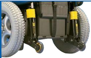
The Rubber Element Suspension is designed to absorb significant jolts and impacts. Standard on the Invacare® Ranger™ X, Torque™ SP and Torque™ 3 Wheelchairs.
