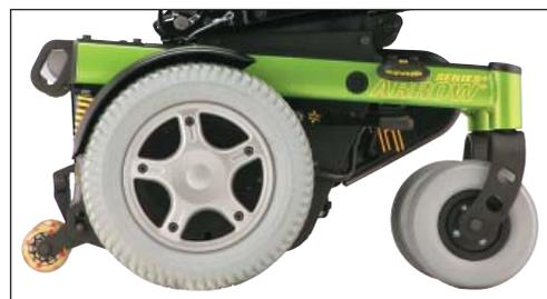
\* TRRO includes four factory-installed transport brackets and a wheelchair anchored pelvic belt. TRRO has been crash-tested in accordance with ANSI/RESNA WC Vol 1. Section 19 Frontal Impact Test requirements for wheelchairs with a 168 lb. crash dummy, which corresponds to a person with a weight of 114 to 209 lb.
