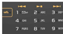
When the Walkman® player, the Radio or the Video player is launched, symbols light up showing the new functions of the top three keys on the keypad.
