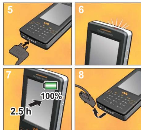
5. Connect the charger, with the symbol on the charger plug facing upwards.
