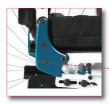
The back angle is adjusted simply by loosening a button-head screw and rotating an adjustment square located on the inside of this back bracket.
