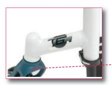
Two pressed bearings located in the fork allow for a more controlled rotation and help to eliminate flutter. The T6A also eliminates problematic caster angle adjustment with our seat frame above the side frame design.
