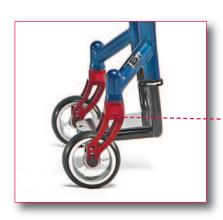
Each custom frame is built to accommodate a short front fork to reduce overall caster trail and keep the user's center-of-gravity low to the ground for improved balance.
