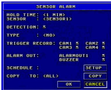
Fig 3.12 Sensor Alarm Configuration
