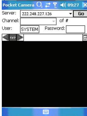
**STEP6** Input the server’s address, ID, and password respectively in the columns of “Server”, “User”, and “Password”. Then click “Go” to login to the DVR. It will show the picture if accessed successfully.
