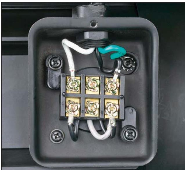
Figure 66. Bandsaw motor wiring.
