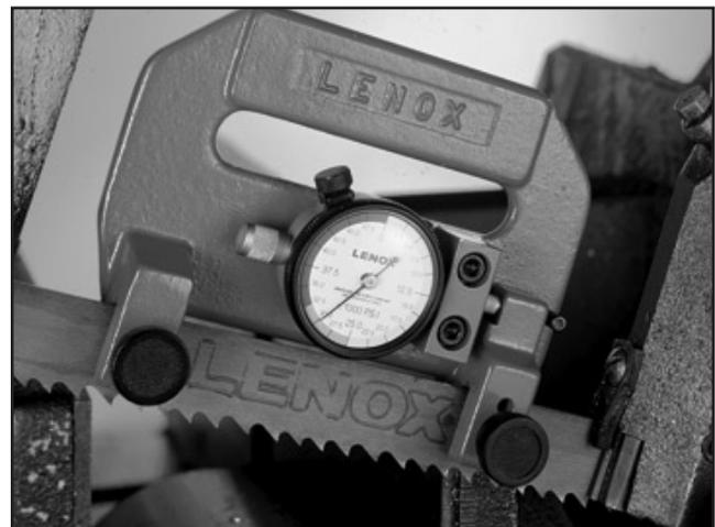
Figure 51. H5408 Blade Tensioning Gauge.
