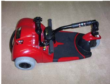
Loosen lock at base of seat post so the battery box can be removed.
