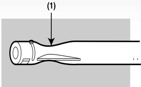
The burner tube air shutter is fitted with a stainless steel screen(1) to prevent spiders and other insects access to the burner tubes through the air shutter openings.
