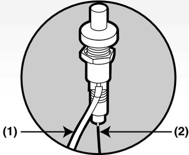
■ Check that the Crossover Ignition button pushes the igniter (button) down, and returns to the up position.
