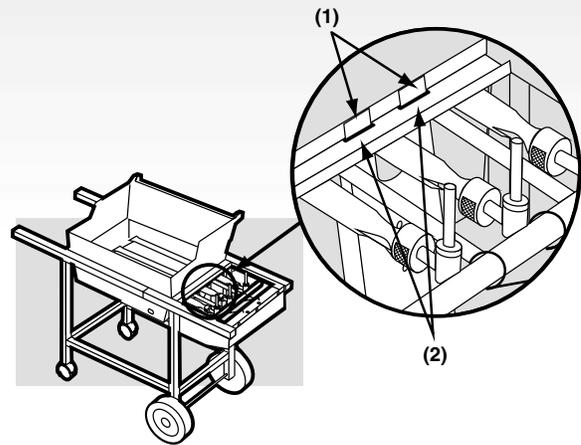
Slide the cylinder panel up until notch at bottom of panel fits over the cross brace(1). Add nylon washer to bolt and insert through the hole in the wheel frame at the bottom right of the cylinder panel, make sure that the bolt slips through the hole in the cylinder panel. Add nylon cylinder glide to bolt end and tighten bolt with the wrench, while holding the cylinder glide with the pliers. Repeat procedure with the hole on the bottom left side of the cylinder panel.
