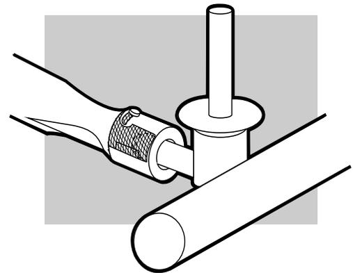
**⚠ WARNING:** After reinstalling the gas lines, they should be leak checked with a soap and water solution before using the barbecue. (See Step: "Check for gas leaks.")
