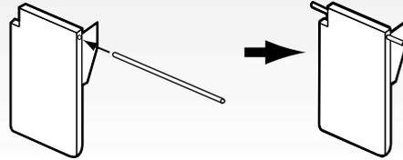
3.) Insert one end of the swing-up work surface rod into the hole in the frame.
