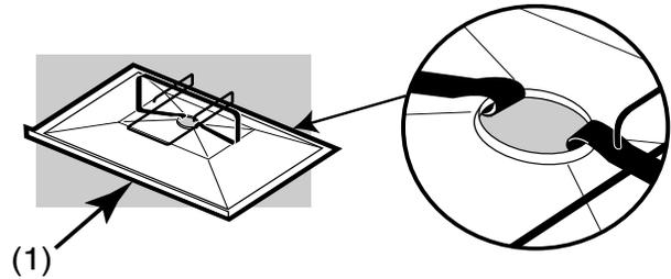
Slide the bottom tray onto the mounting rails under the cooking box with finger grip toward you(1).
