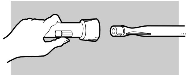
Clean the inside of the burners with a wire (a straightened-out coat hanger will work). Check and clean the air shutter opening at the ends of the burners. Check and clean the valve orifices at the base of the valves. Use a brass bristle brush to clean outside of burners. This is to make sure all the burner ports are fully open.
