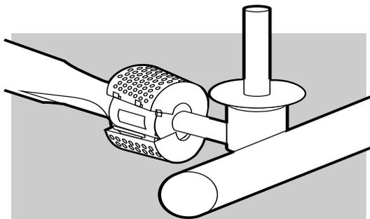
The Weber Spider Stopper™ Guard(1) is factory installed. It fits tightly around the air shutter section of the burner tube and the valve, thereby preventing spiders and other insects access to the burner tubes through the air shutter openings.
