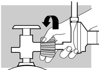
*Note: This is a new type of connection. It tightens clockwise and will not allow gas to flow unless the connection is tight. The connection requires tightening by hand only.*
