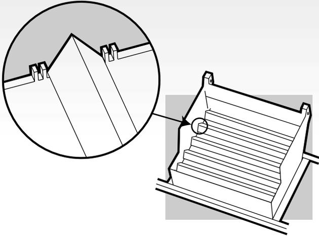
Set the cooking grates onto the ledges in the cooking box with the rounded sides up.
