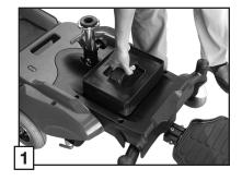
2. Install the seat on the base as shown at right, while pulling the seat rotation lever to lock it in place. Ensure that the seat is locked into place and facing forward before continuing.
