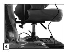
⚠ WARNING: Ensure that the hand control extension is locked in place, and that all cables are away from moving parts of the wheelchair, before occupying or operating
