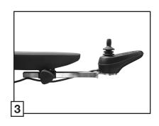
4. Connect the hand control connector to the cowl connector, as shown at right.
