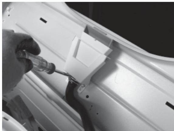
6. Remove hose clamp and Flume/Diverter Hose.
