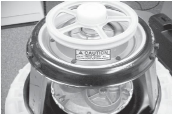
The Brake assembly, as well as the Snubber, is held in position by the Brake Stator which is secured to the underside of the Suspension Housing by six (6) mounting screws.
