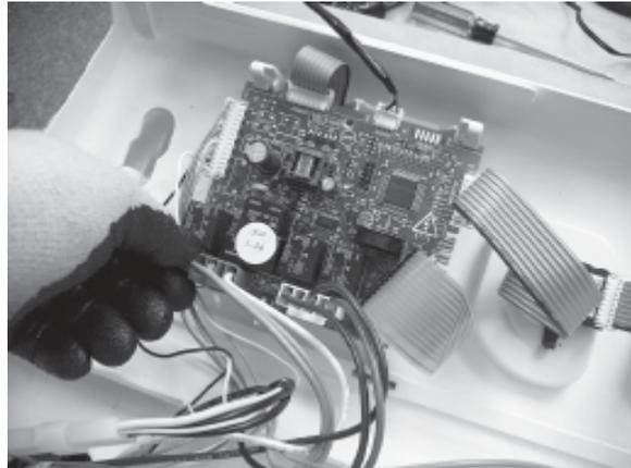
6. Depress the PCB locking tab and remove Circuit Board.
