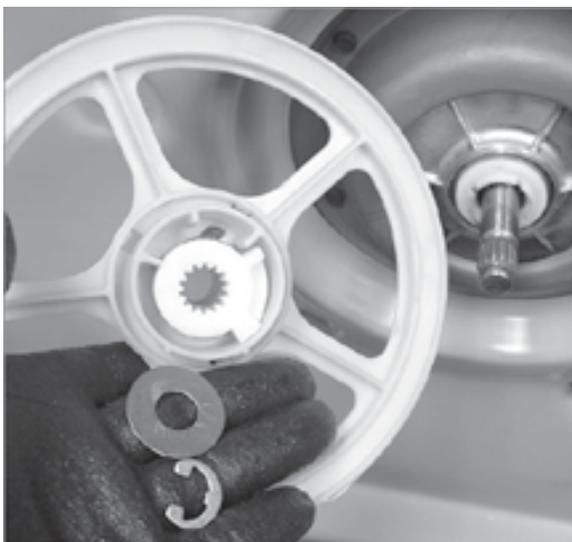
Models are equipped with a plastic Drive Pulley which has the upper Cam molded onto the bottom of the Hub. The purpose of the Pulley and Cam arrangement is to drive the Clutch assembly during the agitate and spin cycle, and to disengage the Brake assembly during the spin cycle.
