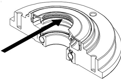
Apply grease to location indicated with arrow on Triple Lip Seal.
