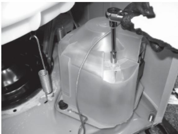
6. Remove Motor wire harness connector.
