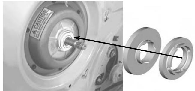
2. Apply a thin layer of **grease** between the contacting surfaces of the Lower Cam and the Drive Pulley.
