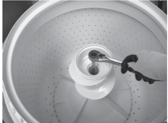
7. Remove Agitator Auger from Agitator Base.
