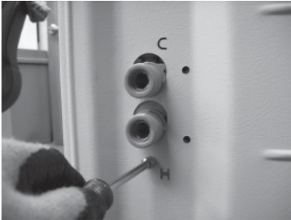
4. Lift Water Valve to align with cutout in back cabinet.
