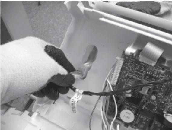
5. Disconnect all wiring harness connectors from the Circuit Board.
