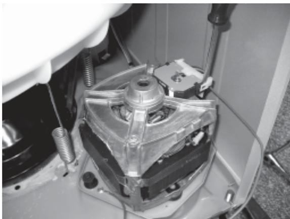
7. Remove three screws retaining Motor to Base.
