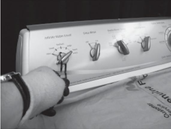
3. Remove three screws along the top of the Console and roll the Console forward.
