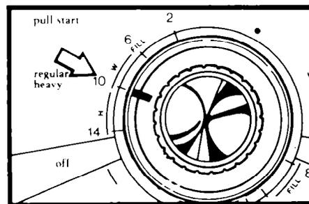
**WARM WATER** can be selected by turning the Control Knob to 8 or 10 minutes in the REGULAR HEAVY Cycle.
