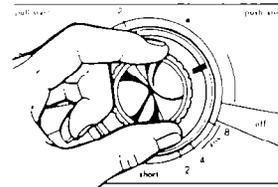
**3.** Set the washer for a DRAIN and SPIN (see page 8). Let it run for about 30 seconds to mix the antifreeze and water.
