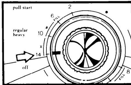
**HOT WATER** can be selected only in the REGULAR HEAVY Cycle. Turn the Control Knob to 12 or 14 minutes in the REGULAR HEAVY Cycle.
