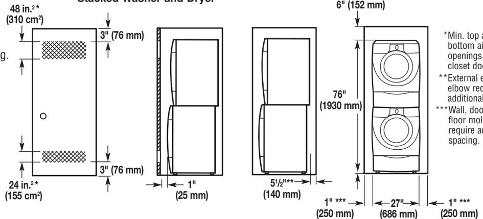
\*Min. top and bottom air openings for closet door.
