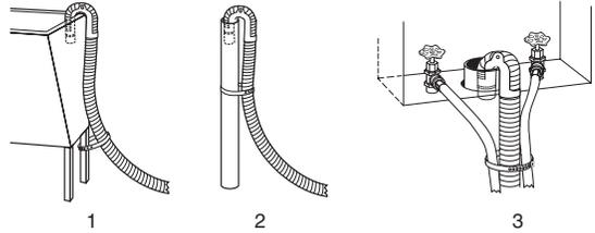
If the washer faucets and the drain standpipe are recessed (see illustration 3), put the hooked end of the drain hose in the standpipe. Tightly wrap the beaded strap around the water inlet hoses and the drain hose.
