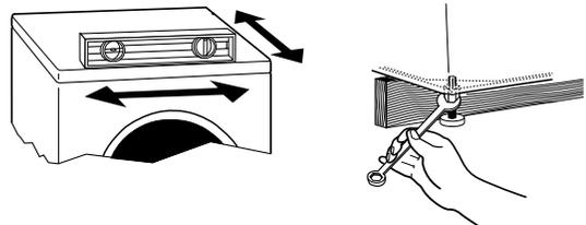
If the washer is against a wall, move the washer out slightly before tipping back. If the washer is not level, first prop the front with a wood block (2" x 4") and adjust the feet as necessary; then prop the back and adjust feet as necessary. Repeat this step until washer is level.
