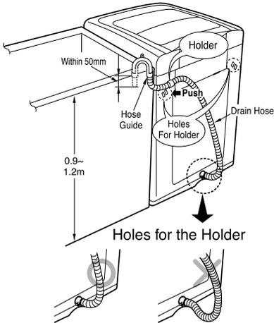
1. Fit the machine end of the drain hose to the outlet of the drain pump and tighten the clamp.
