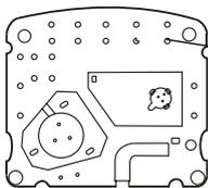
Ventilation hole at the bottom of the washing machine
