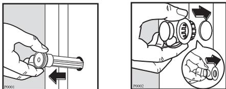
3. Place the machine in an upright position and remove the three plastic bolts.
