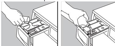
If required, pour fabric softener into the compartment marked
