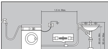
**IMPORTANT:** The distance from the floor to the highest part of the hose should be between 60 to 90 cm. (It is advised to be between 60 and 70 cm). The hose must not be bent nor twisted to avoid clogging. Should a prolongation of the discharging hose be unavoidable this must never surpass 1.5 m and must be of the same diameter as the original hose. Make sure the hoses are not too tense.
