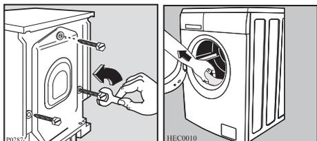
1. Unscrew and remove the three rear screws by means of a key.
