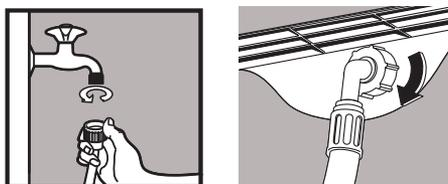
2. If necessary turn the hose adequately by unscrewing the nut at the rear of the appliance. Now tighten the nut anew to avoid leaks. (Open the tap and assure that it does not leak and close it again.)
