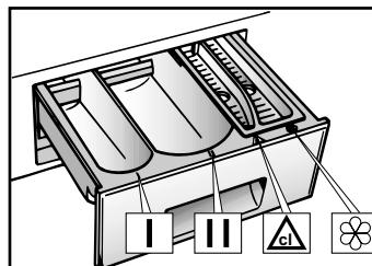
If liquid detergents are used, please insert the special container supplied into the compartment marked "II" in the detergent drawer. This ensures that the liquid detergent enters the drum at the right stage of the wash cycle.
