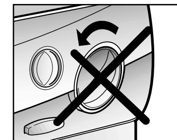
**IMPORTANT : IF YOU NEED TO CHANGE A PROGRAMME THAT HAS ALREADY STARTED – SWITCH OFF THE MACHINE BY THE ON / OFF BUTTON AND THEN MOVE THE PROGRAMME DIAL TO THE CORRECT POSITION. IF YOU DO NOT PRESS “OFF” BEFOREHAND, THE DIAL WILL AUTOMATICALLY MOVE TO ITS INITIAL POSITION.**
