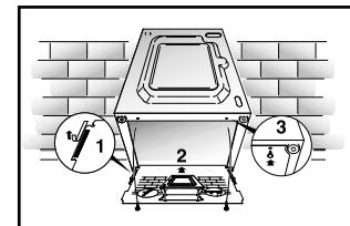
Apply the insulation sheet of corrugated material to the base as shown.
