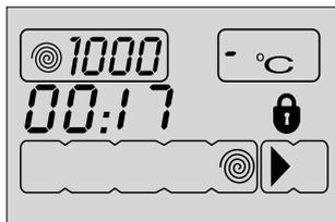
When the “Temperature” button is pressed after coming to the Cold selection, the maximum temperature of the program you have selected will be displayed.
