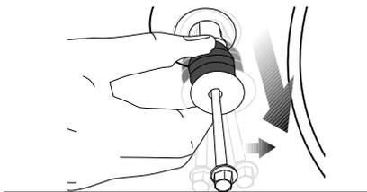
3. Fit the covers (supplied in the bag with the Operation Manual) into the holes on the rear panel. ("P")
