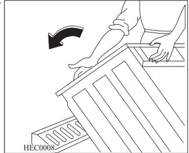
2. Remove the power supply cable and the draining hose from the hose holders on the rear of the appliance.
