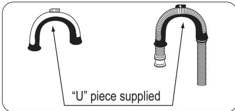
Place the drain hose into your standpipe, which should have an internal diameter of approximately 38 mm thus ensuring there is an air break between the drain hose and standpipe.
