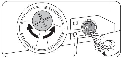
Check carefully whether the pump impeller rotates (it rotates jerkily). If it doesn't rotate, please contact your Service Centre.
