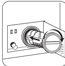
Replace the filter into the pump by inserting it correctly into the special guides. Screw the pump cover firmly by turning it clockwise.
