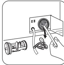
Remove foreign bodies and fluff from the filter seat and from the pump impeller.
