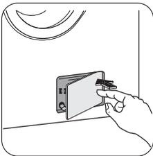
Open the pump door. Place a container close to the pump to collect any spillage.
