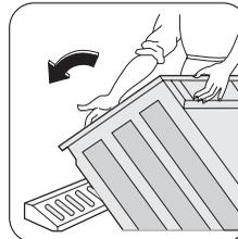
After removing all the packaging, carefully lay machine on its back to remove the polystyrene base from the bottom.
