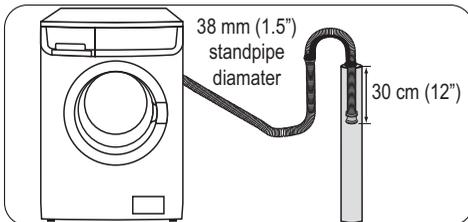
The drain hose may be extended to a maximum of 4 metres. An additional drain hose and joining piece is available from your local Service Force Centre. The joining piece must have an internal diameter of 18 mm.
