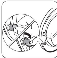
To **activate** this device, rotate the button (without pressing it) inside the door clockwise until the groove is horizontal. If necessary use a coin.
