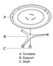
The turntable can rotate in either direction to help cook food more evenly. Do not operate the oven without having the turntable in place. See "Assistance or Service" to reorder any of the parts.
