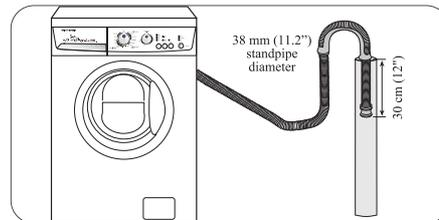
Firstly form a hook in the end of the drain hose using the «U» piece supplied. Place the drain hose into your standpipe, which should have an internal diameter of approximately 38mm thus ensuring there is an air break between the drain hose and standpipe.
