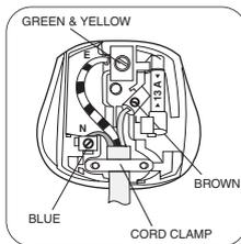
The wire coloured green and yellow must be connected to the terminal marked with the letter «E» or by the earth symbol
