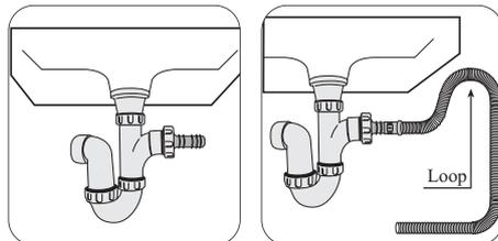
Push the drain hose onto the spigot and secure with a clip if required, ensure a loop is formed in the drain hose (see diagram) to prevent waste from the sink entering the washing machine.
