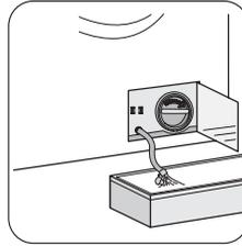
Pull out the emergency emptying hose, place it in the container and remove its cap.
