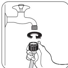
Connect the hose to a tap with a 3/4" thread. Always use the hose supplied with the appliance.
