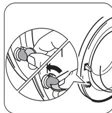
To **disable** this device and restore the possibility of closing the door, rotate the button anti-clockwise until the groove is vertical.
