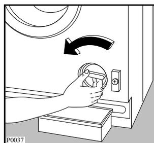
Unscrew and remove the filter.
