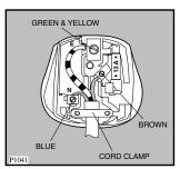
The wire coloured green and yellow must be connected to the terminal marked with the letter  $\ll E \gg$  or by the earth symbol  $\perp$  or coloured green and yellow.
