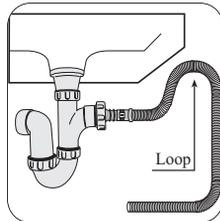
Push the drain hose onto the spigot and secure with a clip, ensure a loop is formed in the drain hose (see diagram) to prevent waste from the sink entering the washing machine.
