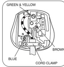
The wire coloured green and yellow must be connected to the terminal marked with the letter «E» or by the earth symbol  $\equiv$  or coloured green and yellow.
