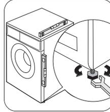
Any necessary adjustment can be made with a spanner. Accurate levelling prevents vibration, noise and displacement of the
