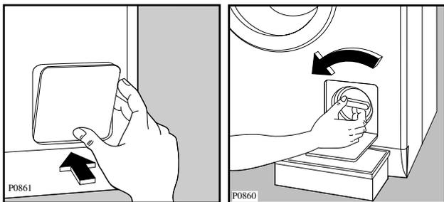
Unscrew and remove the filter.
