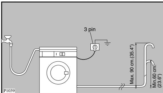
The appliance drain hose should hook into a standpipe, the hook in the drain hose is formed using the plastic "U-Piece" supplied.
