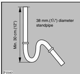
When discharging into a standpipe ensure that the top of the curve in the hose end is no more than 90cm (35.4") and no less than 60cm (23.6") above floor level. The upright standpipe should have a minimum length of 30cm (12") from the bottom of the elbow to the top of the pipe (see diagram).
