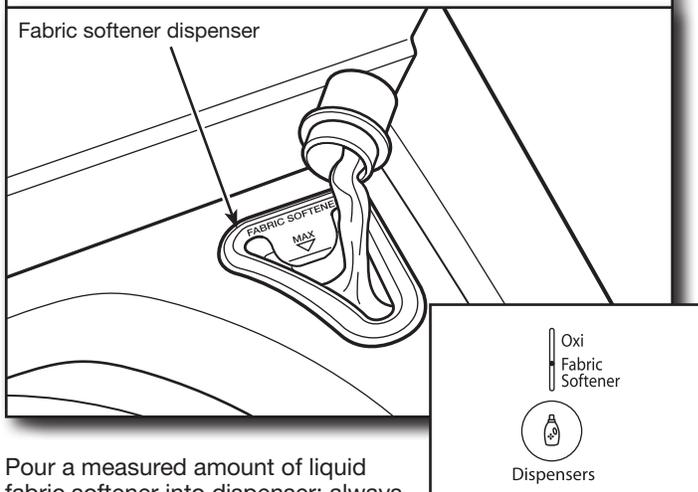
Pour a measured amount of liquid fabric softener into dispenser; always follow manufacturer’s directions for correct amount of fabric softener based on your load size. Then select Fabric Softener option using the Dispensers button.
