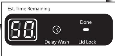
Turn cycle knob to choose your wash cycle. Estimated Time Remaining will light up with a cycle time. You may notice time adjusting during the cycle. This is normal.
