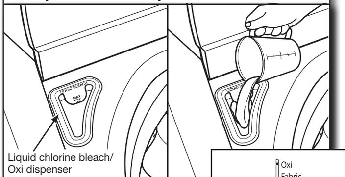
Add liquid chlorine bleach or Oxi laundry boost product to the dispenser. When using Oxi products or other laundry boosters (liquid or powdered color-safe bleach), select the Oxi option, press the Dispensers button until Oxi is selected. It is not necessary to select the Oxi option when using liquid chlorine bleach.
