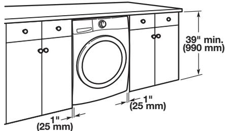
All dimensions show recommended spacing allowed, except for closet door ventilation openings which are the minimum required.
