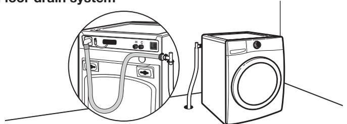
Floor drain system requires a Siphon Break Kit (Part Number 285834), 2 Connector Kits (Part Number 285835), and an Extension Drain Hose (Part Number 285863) that may be purchased separately. See "Alternative Parts". Minimum siphon break height: 28" (710 mm) from bottom of washer. (Additional hoses may be needed.)
