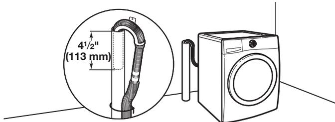
Minimum diameter for a standpipe drain: 2" (51 mm). Minimum carry-away capacity: 17 gal. (64 L) per minute. A ¼" (6 mm) diameter to 1" (25 mm) diameter Standpipe Adapter Kit is available (Part Number 3363920). Top of standpipe must be at least 30" (762 mm) high; install no higher than 96" (2.44 m) from bottom of washer. If you have an overhead sewer and need to pump higher than 96 inches, a sump pump and associated hardware are needed. See "Alternative Parts".
