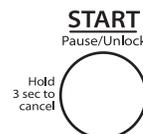
Press the START/Pause/Unlock button to start the wash cycle. Filling is delayed for several minutes while load balance is sensed. When the cycle has finished, the DONE indicator will light. Promptly remove garments after cycle has completed to avoid odor, reduce wrinkling, and rusting of metal hooks, zippers, and snaps.
