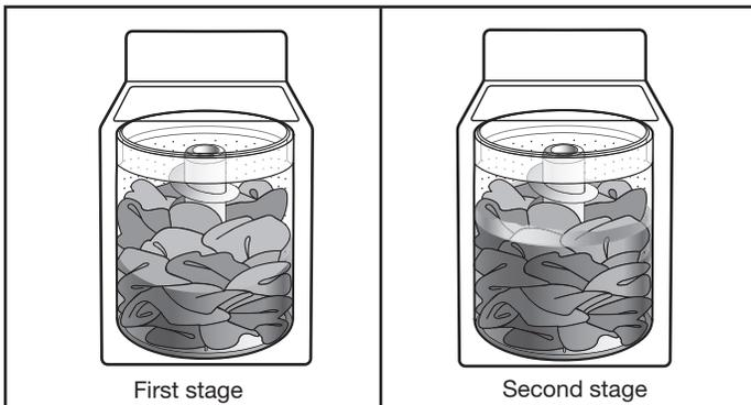
Your new Energy Star® qualified washer saves energy by using lower water levels and reduced wash temperatures, as compared to traditional top-load washers. During the first stage of the wash cycle, it is normal for some of the load to be above the water line. The second stage adds the correct amount of water based on the load size. This washer automatically adjusts the water level to the load size - no water level selector is needed.
