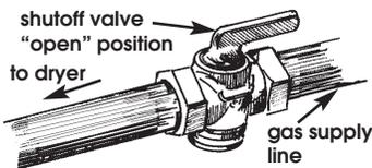
**F.** The supply line shall be equipped with a shutoff valve installed within 6 ft. (1.8 m) of dryer in accordance with the National Fuel Gas Code, ANSI Z223.1 — latest edition\*. In Canada, an individual manual shutoff valve must be installed in accordance with the B149 installation codes CAN/CGA B149.1 and CAN/CGA B149.2\*. This valve should be located in the same room as the dryer and should be in a location that allows ease of opening and closing. Do Not block access to the shutoff valve.
