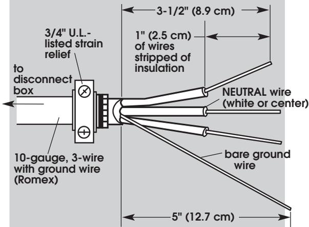
Strip 5" (12.7 cm) of outer covering from end of cable. Leave bare ground wire at 5 inches (12.7 cm). Cut 1-1/2" (3.8 cm) from 3 remaining wires. Strip insulation back 1 inch (2.5 cm).
