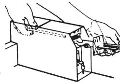
For dryers using coin slides, use adapter kit supplied with dryer.
