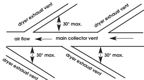
**Back-draft Damper Kits**, Part No. 3391910, are available from your Whirlpool dealer and should be installed in each dryer's exhaust vent to prevent exhausted air from returning into the dryers and to keep the exhaust in balance within the main exhaust vent. Unobstructed air openings are required.
