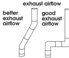
**Four-inch (10.2 cm) metal exhaust vent** is required. Plan installation to use the fewest number of elbows and turns.
