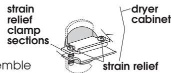
**3. Assemble 3/4" U.L.-listed strain relief (U.L. marking on strain relief) into the hole below terminal block opening. Tighten strain relief screws just enough to hold the two clamp sections together. Install power supply cord/cable through the strain relief.**
