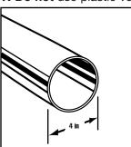
Use 4-inch heavy metal or flexible metal vent. Do not kink or crush flexible metal vent. It must be completely extended to allow adequate exhaust air to flow. Check vent after installation. Refer to your Installation Instructions for proper
