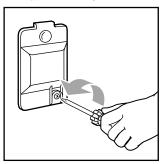
cover from the back wall of the dryer by removing the screw located in the lower right corner of the cover.
