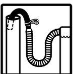
Is the drain hose higher than the water level in the washer? It must be higher for proper operation.
