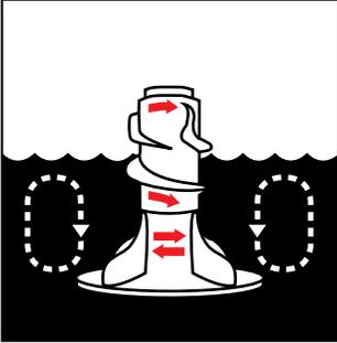
agitator that provides maximum cleaning for all types of washable fabrics. The agitator creates a continuous rollover action that keeps clothes moving
