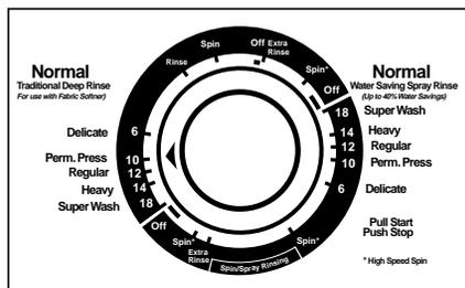
**9. Push in the Cycle Control Knob and turn it clockwise to the Normal cycle you want.**
