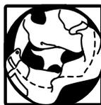
Load evenly to maintain washer balance. An off-balance load can make the washer vibrate during spin.
